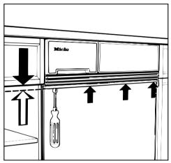
The attached adapter strips can be compressed up to 3/8" (10 mm) by tightening the 4 nuts located under the bottom adapter strip. If the control panel needs to be shortened by more than 3/8" (10 mm), one or more adapter strips can be removed.
